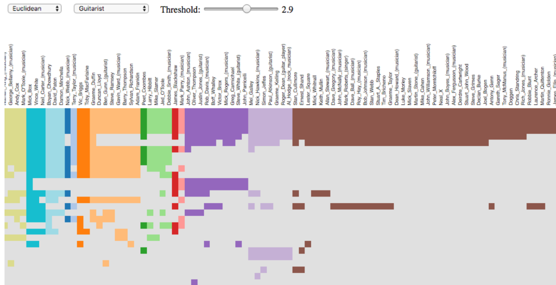
Figure 7.5: A zoomed portion of the matrix showing the results of the hierarchical clustering algorithm performed on the elements of some classes of DBpedia. Instances are placed on the columns while predicates on the rows. Each column is a vector describing an instance in term of predicates. Similar instances are kept close and depending on the threshold coloured according to the results of the clustering process. An interactive version of this visualization can be consulted at http://bl.ocks.org/fabioalse/cc44f1a671e3ce135775 .
